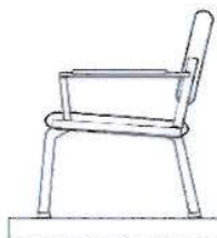
Figure 4c - Type III - Fixed seat angle, fixed backrest Types of Chairs
